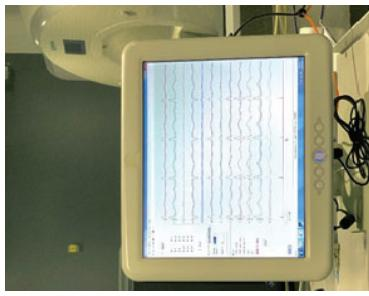
The CRM must be installed in the MRI control room in a hospital environment. Under no circumstances should the CRM be placed in the MRI room as it is not MRI safe. Place the Control Room Monitor on a desk-top where the user can see the display to monitor the patient's ECG. A mouse and monitor touch screen pointer are provided to ease operation of the monitor.
